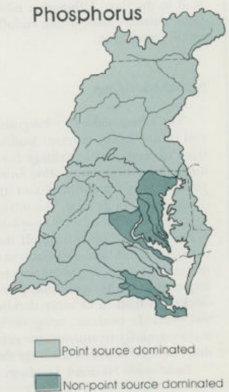
Importance of point or non-point sources for phosphorus in the major drainage basins.
