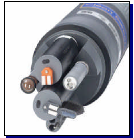
An instrument similar to the one pictured above is lowered through the water at 150 stations throughout Chesapeake Bay. The sensors on the instrument measure DO, temperature, salinity and several other water quality parameters.
