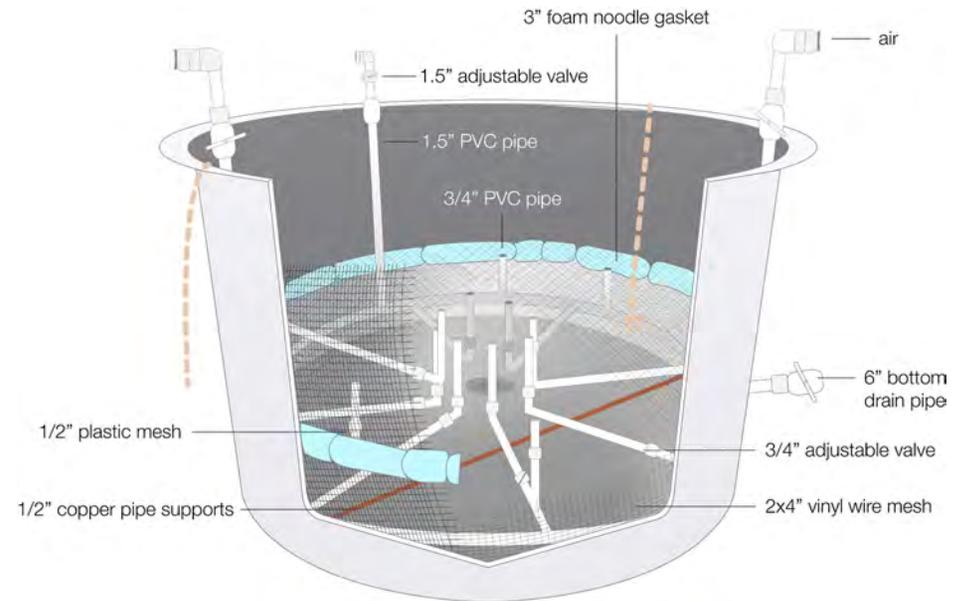
Figure 29 - Schematic of the Turbulator.
